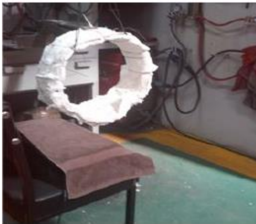
Fig. 4. Pipe coupons covered with a 12.5 mm thick insulator.
